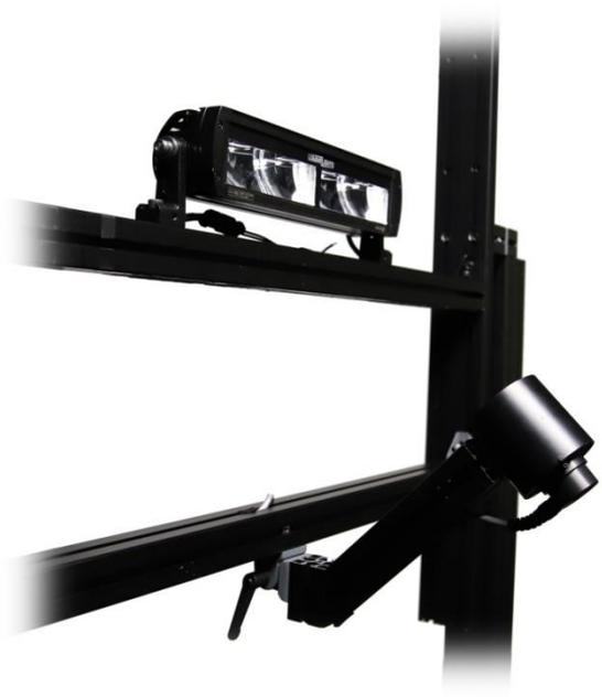
**Fig. 4. SSL BPC-B.** The burning position corrector setup in case of type B goniometer (photo: SSL LUMI 120 goniometer).
