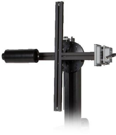
**Fig. 2. SSL BPC-C.** The burning position corrector setup at normalized measurement position ( $E_{measBP}$ ) in case of type C goniometer (photo: SSL LUMI 90 goniometer).
